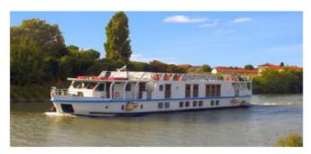
Former purpose: Sand barge on the River Po Year of construction: 1960 21.6ft x 147.6ft (6.6m X 45m) Dimensions: Year converted into a floating hotel: 2010 Generators: AIFO IVECO SRM55M (550 Horse Power x 2) Main engine: Maximum speed: 10 knots 20,000 litres Water capacity: 12,000 litres Fuel capacity: Cruise distance: 174km
