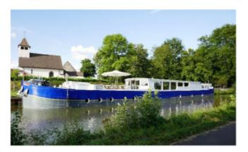
Former purpose: Freight barge from Belgium Year of construction 1950 Dimensions: Length 128ft (39m). Width 16ft 6" (5.03m) Year converted to a Hotel Barge: 2015 / 2016 Generators: 2 x 220 volt generators both equipped with hospital silencers for night running Main Engine: 206kw Scania Maximum Speed: 15 knots Water & fuel capacity: 8000L of water 2000L of fuel
