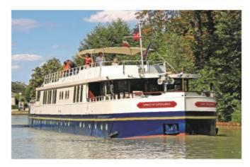
Year of construction:Commissioned in 2003Dimensions:Length 126ft (38.4m) Width 17ft (5.2m)Generators:2Main engines:2 x Volvo PentasMaximum speed:10 knotsWater & fuel capacity:20 tons of water, 6 tons of fuel
