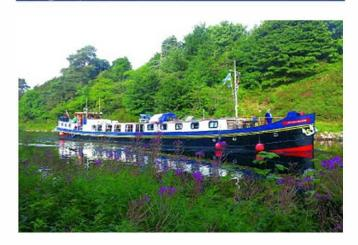
Former purpose: Cargo Barge operating in Holland Original year of construction: 1931 Dimensions: Length 117ft (35.66m) Width 16ft 6" (Sm) Year converted to a Hotel Barge: 2000 Generators: 2 x Cummins Onan 27kva generators Main engine: Gardner 6LX 127HP Maximum speed: 7.5 knots Water & fuel capacity: 8 tons of water and 3 tons of fuel
